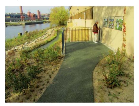
Figure 1. Signs at the viewing platform for the installed wetland and Bronx River inform visitors about how the wetland is cleaning up parking lot runoff and, therefore, protecting the river and also offering habitat to urban wildlife. The railing was salvaged from the old Yankee stadium. Photo by Lillian Ball.
